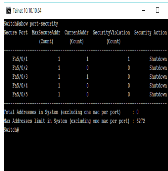
Gambar 10. Tampilan Monitoring Port Security di Command Line
